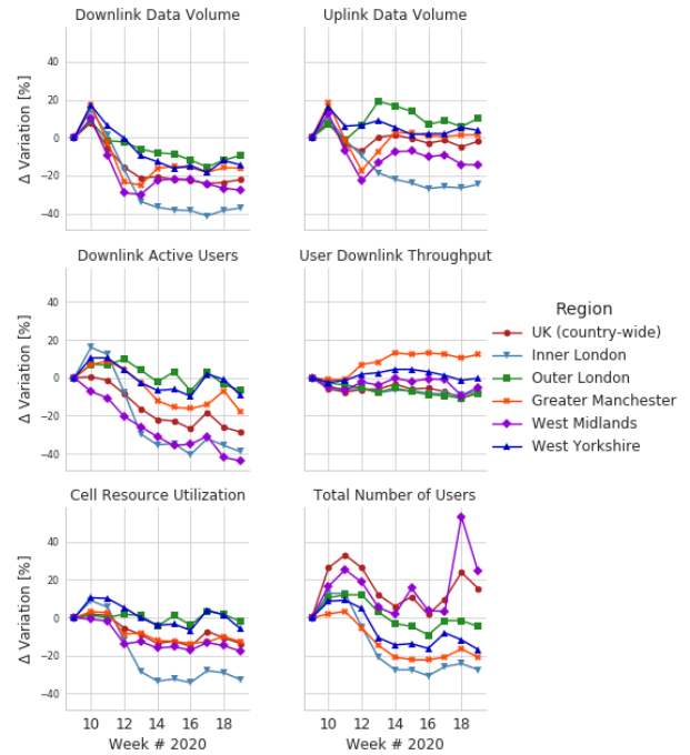
Figure 8: MNO performance characterization, using metrics for all data traffic. Each plot corresponds to a metric, as we indicate in the title of the plot. We show the median values for the delta variation percentage for each metric over one week (each point on the x-axis corresponds to a week #), using as a baseline for comparison the median value in week 9. Each line corresponds to different geo-regions within the UK, including "UK - all regions", which accounts for the entire country.
